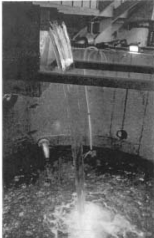
Figure D. Discharge over a horizontal edge (weir), simulating Ringhals 2
