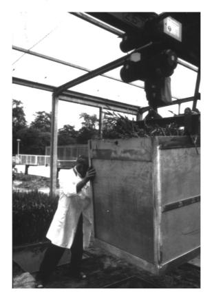
Insertion of a lysimeter casing into the container embedded in the ground of the lysimeter station (top) and total view of lysimeter station (below) (6)
