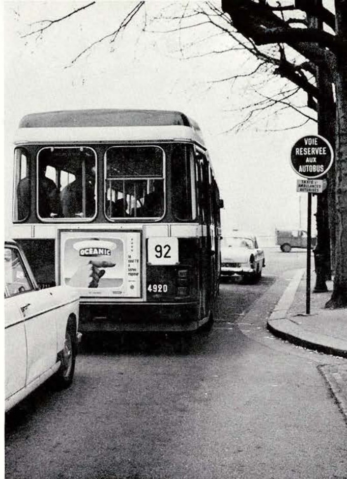
Separating public transport from the rest of the traffic flow by means of exclusive bus lanes.
