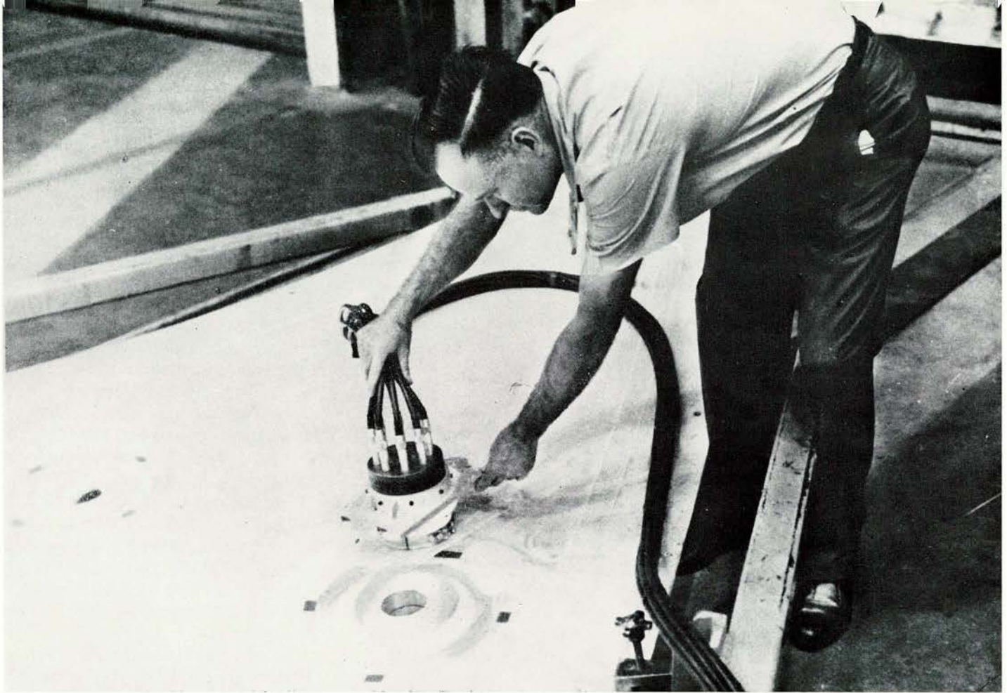
An electromagnetic hammer corrects distortions in metal surfaces through magnetism — one of many space techniques that could change the job profile of the metal worker of the future.
