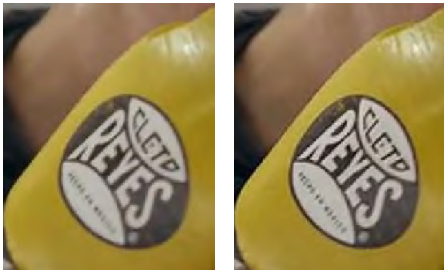
Fig. 15 – Cropped screenshots from an exemplary El Fuente sequence (left: x264 @ 2654 kbps, right: LCEVC @ 2051 kbps)
