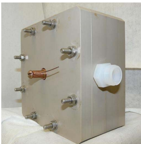
Figure 3: Photograph of the custom-made high flow single-cell electrolysis cell
