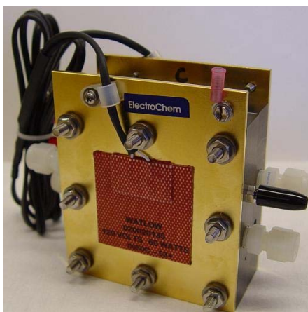
Figure 2: Photograph of the single-cell commercial fuel cell used for low flow CuCl/HCl electrolysis experiments
