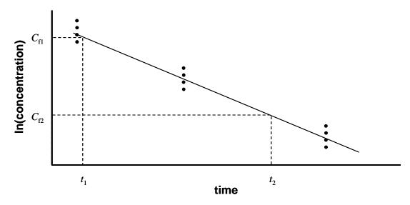
Note that deviations from a straight line may indicate a more complex depuration pattern than first order kinetics. The graphical method may be applied for resolving types of depuration deviating from first order kinetics.
