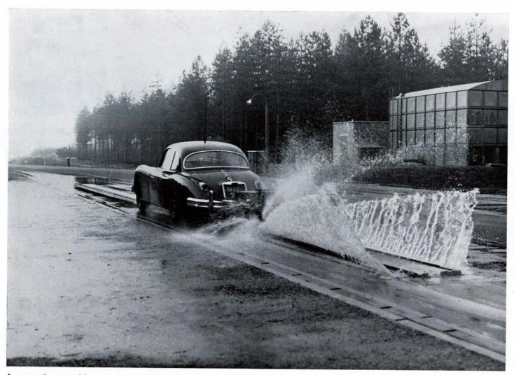
An experiment with a single-wheel trailer passing through a water-trough at high speed (Road Research Laboratory, Harmondsworth, U.K.)
