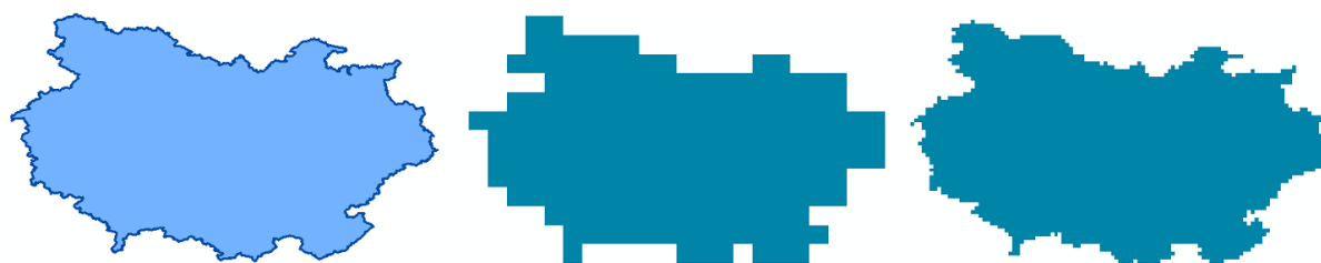
Figure 4. Representation of Paris metropolitan area as a vector, raster at 0.1 degree cells size and raster 0.02 degree cell size (from left to right)
