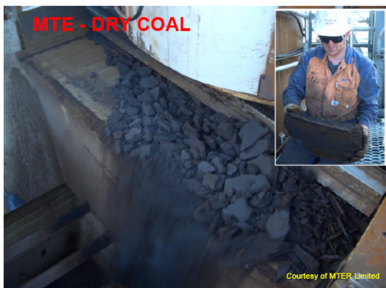
Figure 12 Photograph of the dried product from the 15 t/h MTE Rig
