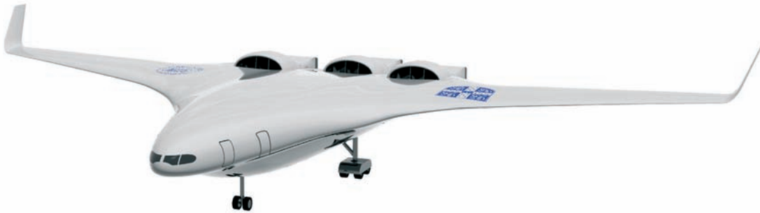
Figure 15.16 ► Blended wing body: SAX-40 design
